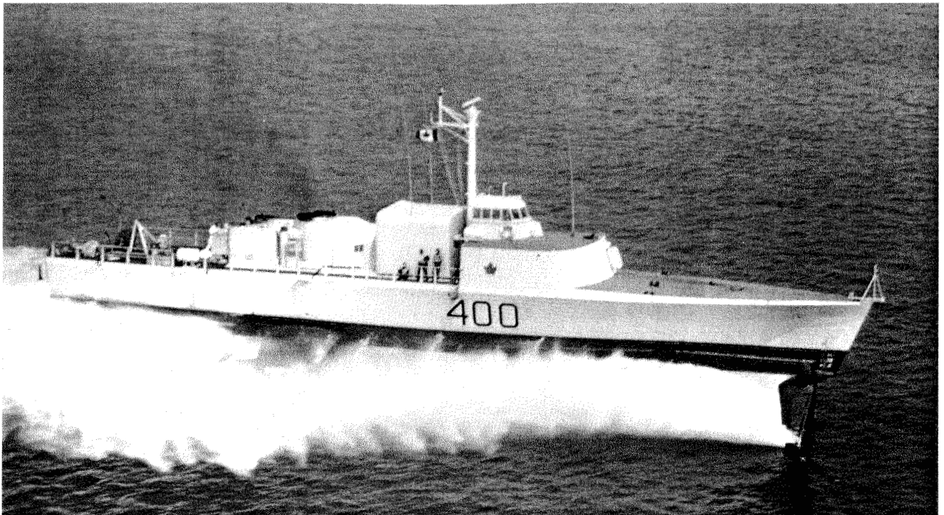
Bras d'Or during a demonstration run in Hampton Roads, 24 June 1971. Official USN Photograph USN K-90232, taken by PH2 Thomas L. Lawson USN. Bras d'Or's foil and power system differs substantially from the submerged foil, water jet system employed by the current U.S. Pegasus (PHM-1) class design.
