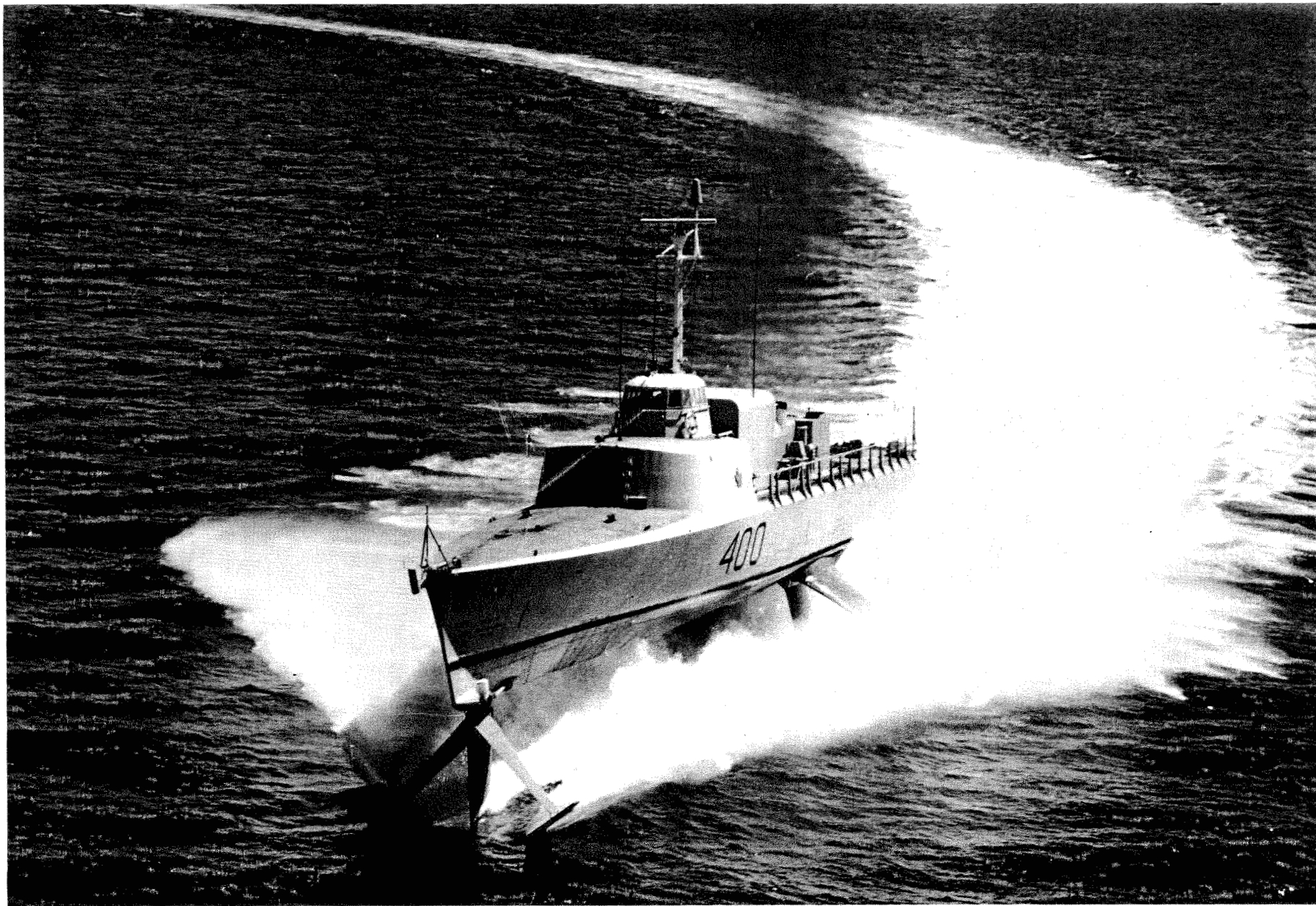
Bras d'Or comes about for a photographer aboard a helicopter. The anhedral foil tips proved their worth, smoothing turns and indeed tightening them. However, they added $1M to the cost and were criticized by experts and press alike. Author's photograph, copyright.
