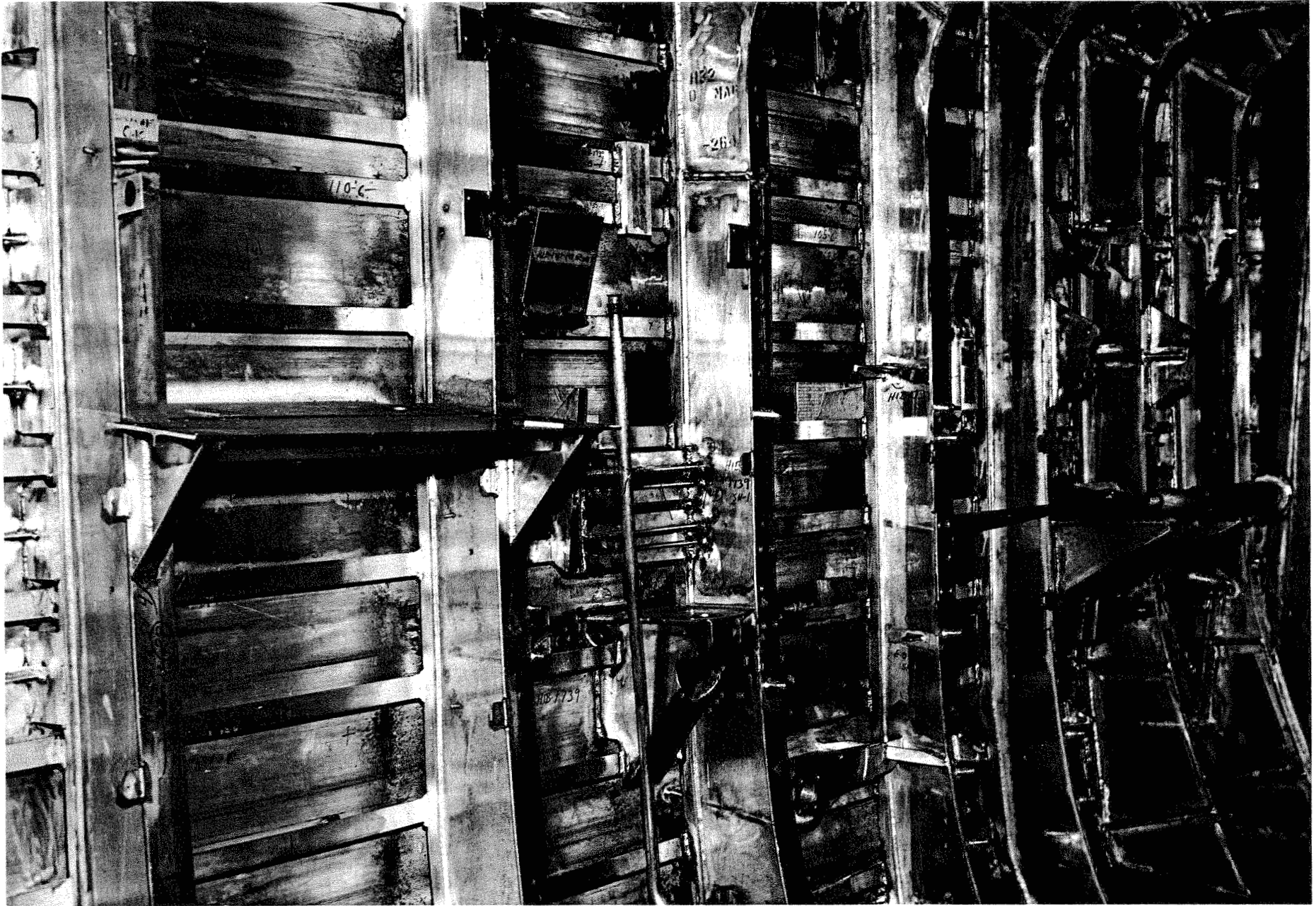
An interior view of the hull—this was a section of the ship that was burned through in the Nov. 1966 fire. The plates and ribs are fabricated from Alcan D54s aluminum. The aluminum was still as shiny as seen here when the author visited the ship in 1979. Author's photograph, copyright.
